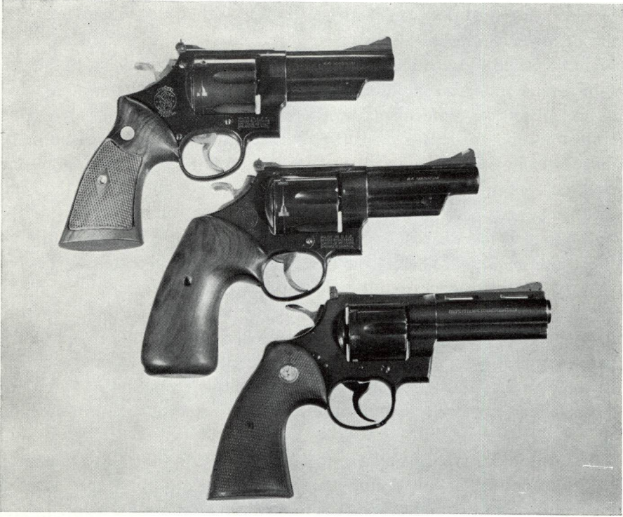
Smith & Wesson target grips (top) and Colt target grips (bottom) showing bulge built into metal at top of grip strap and flared bottom of grips as contrasted to custom grips designed for double action shooting with heavy recoil weapons.
