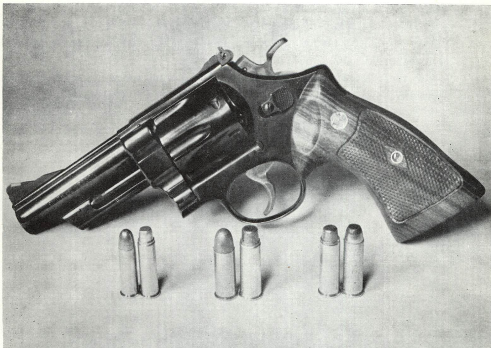
Pictured here is the new S&W Model 57 in .41 Magnum caliber. Loads in foreground from left to right: 38 Special and .357 Magnum; .44 Special and .44 Magnum; .41 Magnum lead and jacketed loads.
