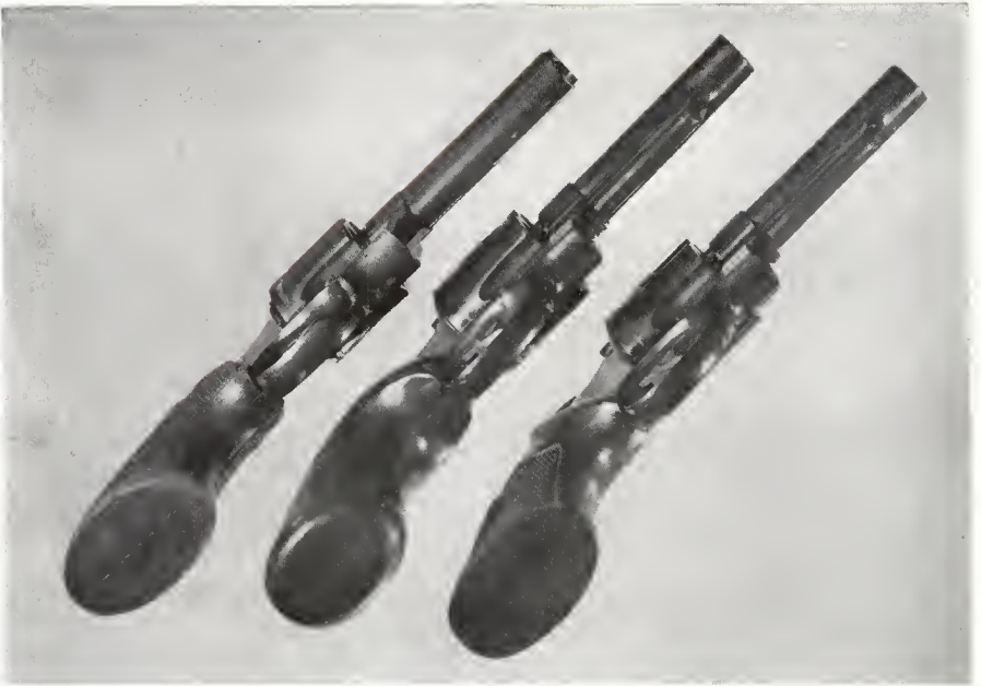
Contrast shown from two angles. Factory grips on left and right, combat style custom grips in center. Note the wide bearing surface of filler on the custom grips as compared to the narrow, rounded surface of the commercial "target" grips.
