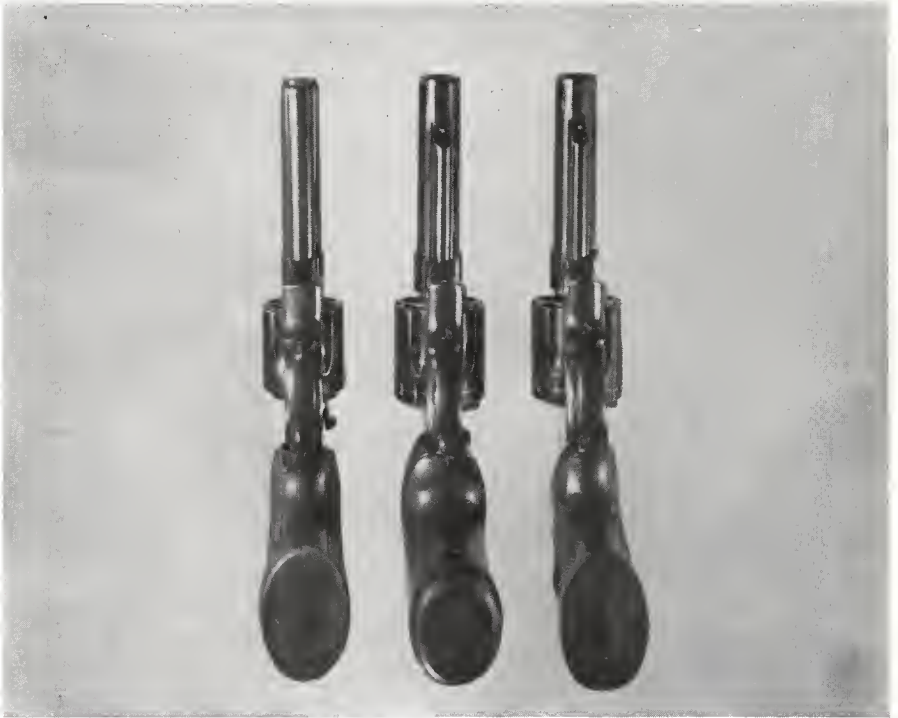
Contrast shown from two angles. Factory grips on left and right, combat style custom grips in center. Note the wide bearing surface of filler on the custom grips as compared to the narrow, rounded surface of the commercial "target" grips.
