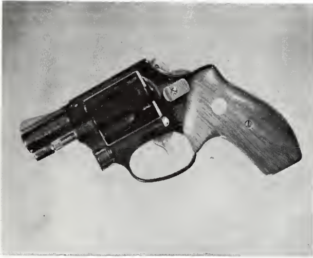
S & W Chief Special Airweight, .38 Spl. caliber. This is a fine hideout gun due to its fire power, small size and negligible weight. Would be ideal in .22 RFM caliber.
