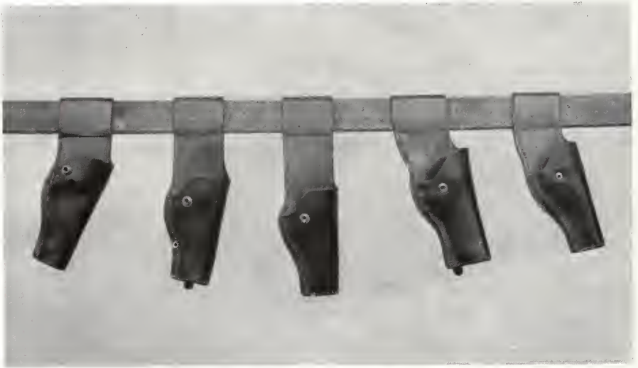
Five different angles of tilt, backward and forward, from the straight drop holster in center. No appreciable difference in speed could be detected after practice with each.
