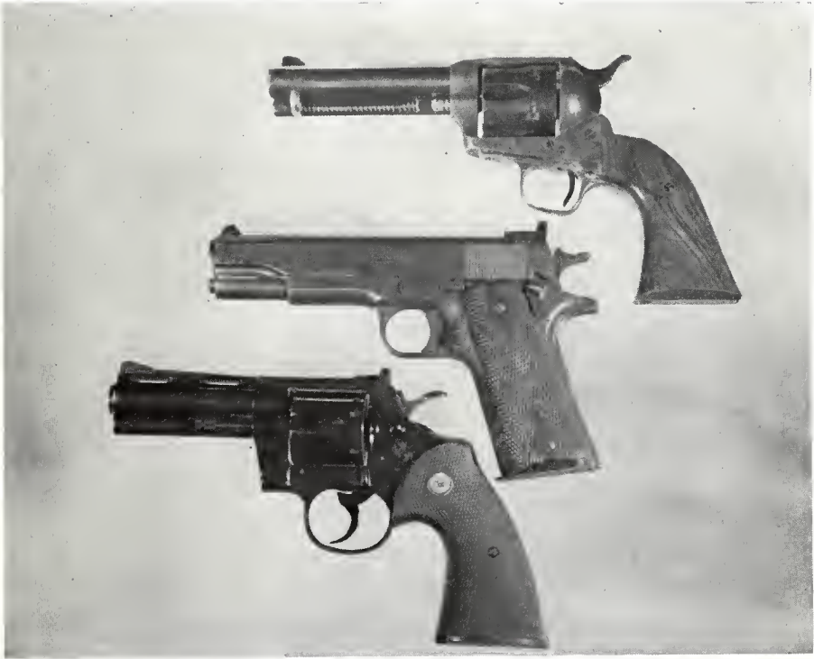
Above: The three basic types of handguns. Reading from top to bottom: Single action; Auto-loader; and Double action. The double action is the type best suited for service use in Law Enforcement.
