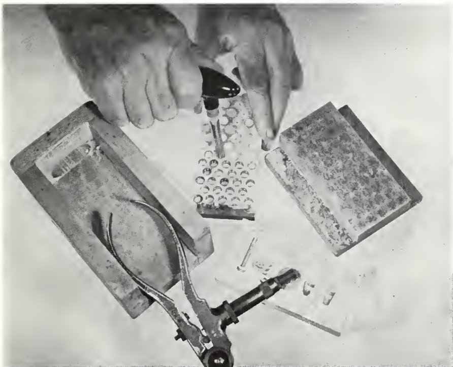
After removing from box, turn over and push paraffin bullets to bottom of case. Cases are then removed and after priming, are ready to shoot.
