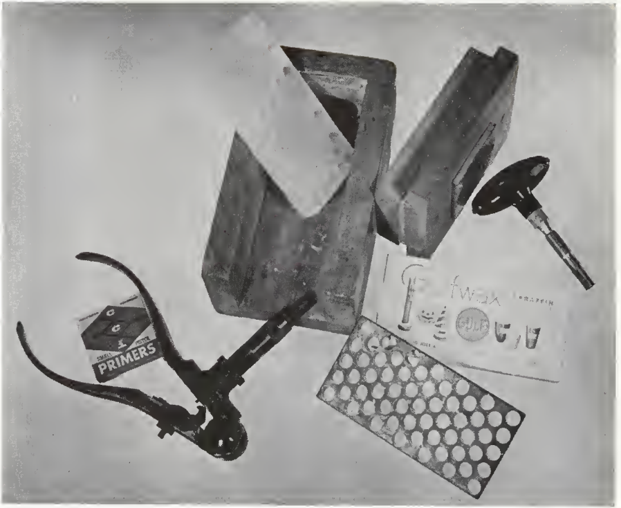
Homemade kit. Cake of wax with perforations has already been used and can be discarded or remelted into cake of proper size.
