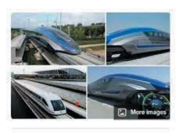
Maglev is a system of train transportation that uses two sets of magnets, one set to repel and push the train up off the track, and another set to move the elevated train ahead, taking advantage of the lack of friction. Wikipedia
